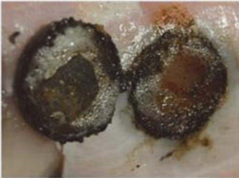
A photograph showing two pieces of chicken meat. The piece on the left has a dark, circular area where the battery was placed, showing significant discoloration and what appears to be a small crater or hole in the meat. |
